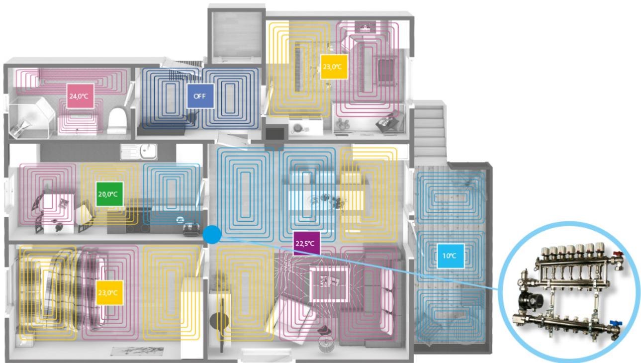
TRITONE overcomes the distinction between advantaged and disadvantaged position rooms. You can set the circuit temperature of the rooms in a very few easy steps. The flow rate supplied by the generator is kept constant in all the rooms.
