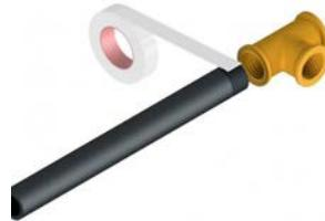
Please check if there isn't an excess of the above mentioned coat, in order to prevent possible breakings caused by excessive screwing.
