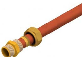
Insert the pipe in the body until it stops and tighten the nut by hand until allowed.
