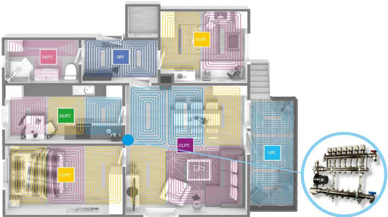
TRITONE overcomes the distinction between advantaged and disadvantaged position rooms. You can set the circuit temperature of the rooms in a very few easy steps. The flow rate supplied by the generator is kept constant in all the rooms.
