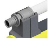
Put pipe and sleeve in abutment.
