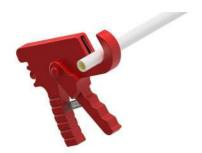
Calibrate the pipe using special reamer [code CS50.00, MA00.90], removing possible residual chips. The pipe edge should be trimmed throughout the circumference.
