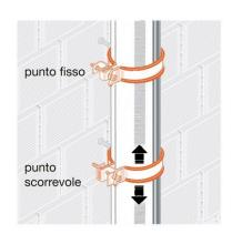
In long sections of straight piping, to absorb any variations in length, it is advisable to insert at least one expansion elbow every 10m of pipe, as shown in the following diagram. For pipes with a diameter equal to or greater than 32mm, the expansion curves are mandatory.
