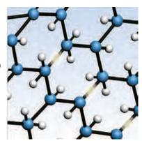
The best and most accurate way of cross-linking polyethylene is through the use of electron beams. Polyethylene can be cross-linked in the following ways:
