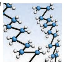
Exposing the multilayer pipe to intense electron beams creates cross connections between the different molecular chains in the plastic. The electrons cause the hydrogen atomsto split from the various polyethylene chains. This enables carbon atoms to bond to each other and form a strong cross-linked structure.
