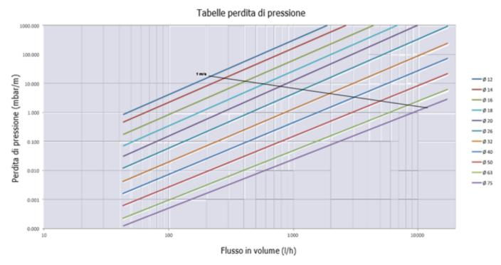
Liquids lose energy when they flow through a pipe as a result of friction between the liquid and the walls of the pipe.
