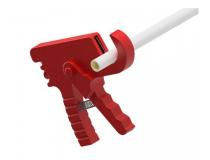
Calibrate and deburr the pipe with a special gauge, taking care to eliminate any residual chips. The internal chamfer must be made on the entire circumference.
