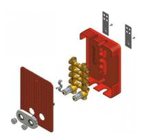
Once the chases have been made on the boarding, the case is walled after attaching the two galvanised steel brackets, positioned on the sides at the top of the case. The manifold is then fixed to the case using a clip and screw (included in the package).
