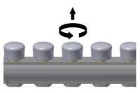
TRITONE does not require balancing the flow rate of the circuits, as it is a constant flow rate control unit. It is however possible to adjust the temperature of each individual circuit.
