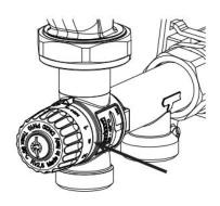
3.Set a mixed water temperature value slightly lower than the design temperature. Activate the generator and wait until it reaches its design working temperature (higher than the valve setting). Activate the group pump. Wait until the mixed water temperature gets stable. Read its value on the flow temperature gauge.
