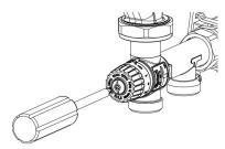
4. Counterclockwise rotate step by step the knob to increase the temperature. Then wait until the temperature gets stable. Read its value on the flow temperature gauge. Proceed in the same way until the design flow temperature is reached.
