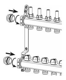
Screw the other side of the fittings to the regulating group, using the running nuts with flat gasket supplied in the package.
