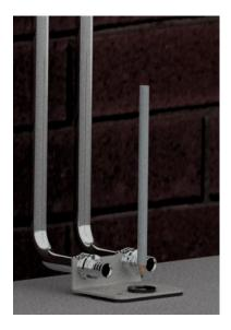
Unscrew the connection kit, remove the pipes and drill the fixing hole of the floor bracket. Insert the gusset into the hole made in the floor.
