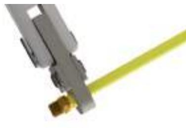
*Place the pressing jaws and operate the electric button of the pressing machine. An improper placing of the jaws could damage the proper system functioning*
