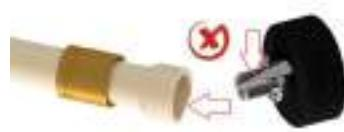
*Cut pipes which are not circular adjust after expansion and waste the piece of non-conformed pipe. Replace expanders which are damaged or do not allow perfect circularity of the enlarged pipe. The defective expander can cause sealing problems over time.*
