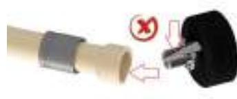
*Cut pipes which are not circular adjust after expansion and waste the piece of non-conformed pipe. Replace expanders which are damaged or do not allow perfect circularity of the enlarged pipe. The defective expander can cause sealing problems over time.*
