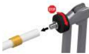
*Check that the expander is not damaged and it is screwed up to the end. Once screwed the expander shouldn't unscrew during the rotation of the pipe on the expander. Verify that the tool we are going to use is correct and studied for the pipe we are going to assemble. Insert the expander without forcing and parallel to the axis of the pipe.*
