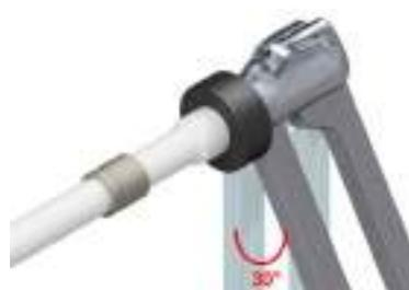
*The expansion operation must be repeated at least a second time by turning the equipment by 30 °. If the internal part of the pipe is not perfectly cylindrical, repeat the described operations again.*
