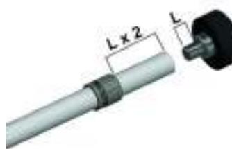
*Insert the sleeve into the pipe, making sure that the marked strip is opposite to the cut of the pipe and that there is double distance compared to the sleeve between the end of the pipe and the sleeve itself.*
