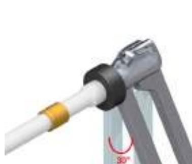
*The expansion operation must be repeated at least a second time by turning the equipment by 30 °. If the internal part of the pipe is not perfectly cylindrical, repeat the described operations again.*
