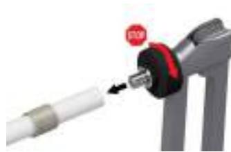
*Check that the expander is not damaged and it is screwed up to the end. Once screwed the expander shouldn't unscrew during the rotation of the pipe on the expander. Verify that the tool we are going to use is correct and studied for the pipe we are going to assemble. Insert the expander without forcing and parallel to the axis of the pipe.*
