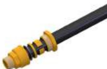
*Insert the components on the pipe according to sequence that follows: nut, cut olive (external surface marks have to be directed forward the nut and not forward the fitting), compression ring and gasket (and at the end the sleeve, where expected).*
