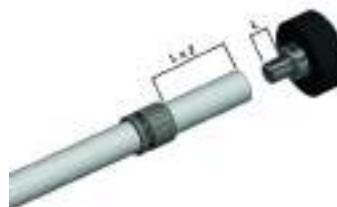
*Insert the sleeve into the pipe, making sure that the marked strip is opposite to the cut of the pipe and that there is double distance compared to the sleeve between the end of the pipe and the sleeve itself.*
